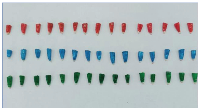
[Table/Fig-9]: Samples coated with nail varnish except 2 mm around the root apex.
